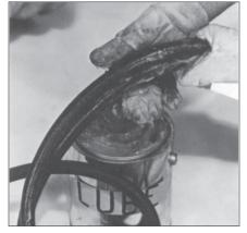
Liberally lubricate gaskets with either a soap-base lubricant such as Tylox 7 Lubricant or a vegetable base lubricant such as Crisco<sup>®</sup>.
