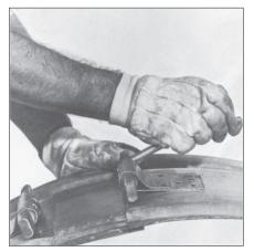
T if necessary, use the bolt to turn the bar so that the holes are in alignment
